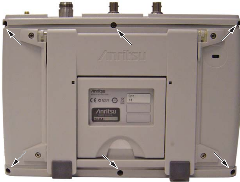
Figure 6-2. Location of Six Screws that Secure Case Back to Case Front
